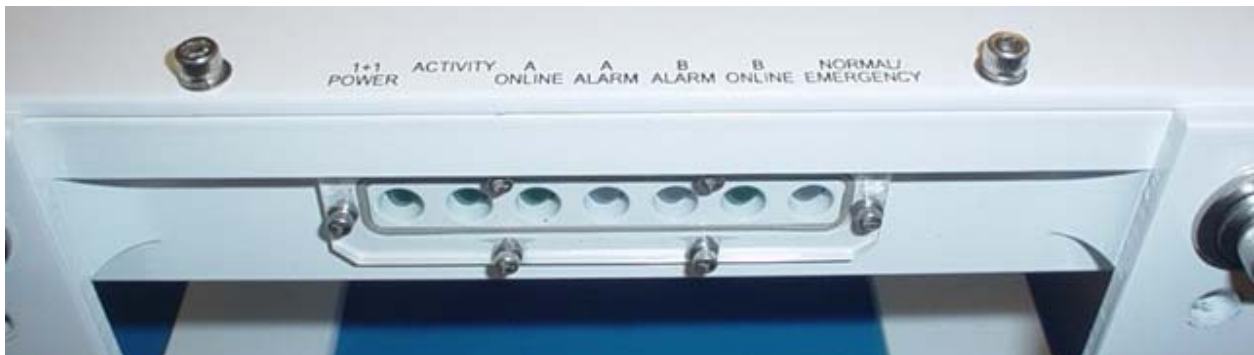
Figure 7-7 RX 1+1 Interface Module Side View
