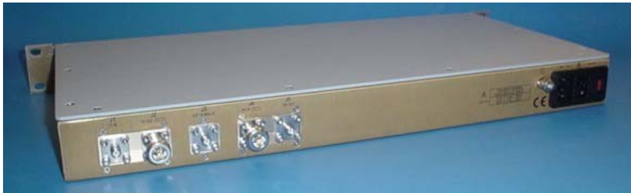
Figure 4-3 IFU Back Panel
