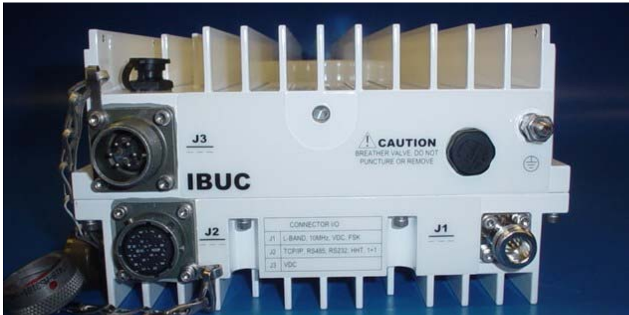
Figure 4-1 IBUC Front Panel
