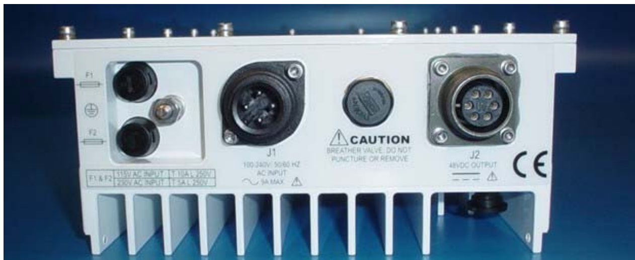
Figure 4-2 PSUI Front Panel
